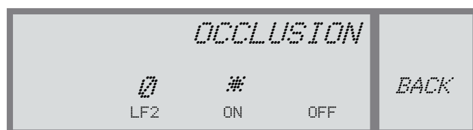
Fig. In the Occlusion manager, gain for the lowest frequency band can be adjusted to solve occlusion problems. LF2 (350-500Hz).
