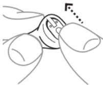
To turn the hearing aid on, close the battery lid and push it upwards. The hearing aid will play a sound signal to indicate that it is on, unless your hearing care professional has deactivated this function.
