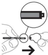
Insert the new wax guard into the opening of the sound outlet and press it gently.
