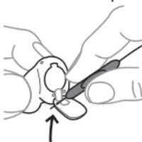
Open the battery lid and turn the hearing aid so the lid is facing downwards (see illustration). Guide the short wax removing tool (no. 4) through the microphone openings on the lid from the inside (see illustration).
