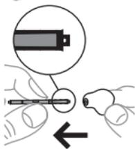
Pull the used wax guard straight out.
