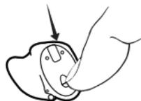
Use the nail grip to push the battery compartment cover downwards and open the cover.
