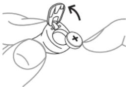
Now place the battery in the drawer as shown. Close the drawer. If it doesn't close easily, the battery is not placed correctly. If you are not using the hearing aid for a few days, remove the battery.
