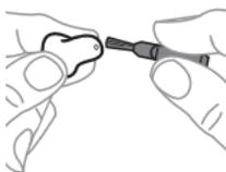
Remove any visible earwax from **around** the sound outlet with the small brush or cloth. **Never** try to clean the wax guard.
