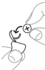
Now place the new battery in the door as shown. Close the door. If it doesn't close easily, the battery is not placed correctly. If you are not using the hearing aid for a few days, remove the battery.
