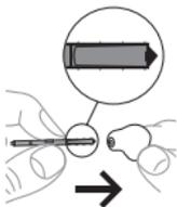
Insert the removal hook into the used wax guard.
