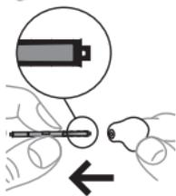
Pull the used wax guard straight out.
