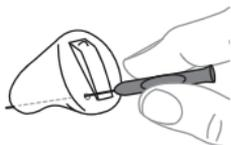
Short vent: clean the vent as far as the long end of the wax removing tool (no. 3) can reach.
