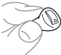
To turn the hearing aid on, close the battery door and push it upwards. The hearing aid will play a sound signal to indicate that it is on, unless your hearing care professional has deactivated this function.
