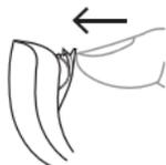
To turn the hearing aid on, close the battery door. The hearing aid will play a sound signal to indicate that it is on, unless your hearing care professional has deactivated this function.
