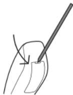
To open battery drawer, use the special tool you've received, and do as illustrated.
