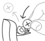
Now place the new battery in the drawer as shown. Close the drawer. If it doesn't close easily, the battery is not placed correctly. If you are not using the hearing aid for a few days, remove the battery.
