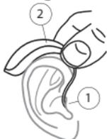
1. Insert the ear-set in the ear while holding the lower part of the tube/earwire. Pulling the outer ear upwards and backwards at the same time can be helpful.
