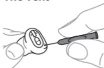
Clean the vent every day by passing the long wax removing tool (no. 4) all the way through the vent.
