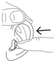
Close the battery lid completely. Hold the hearing aid with your thumb and forefinger and insert it slowly into your ear until you feel resistance. Then use the tip of your forefinger to gently push the hearing aid into your ear until it feels comfortable. Pulling the outer ear upwards and backwards while you insert the hearing aid can be helpful.
