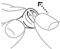
To turn the hearing aid on, close the battery door and push it upwards. The hearing aid will play a sound signal to indicate that it is on, unless your hearing care professional has deactivated this function.
